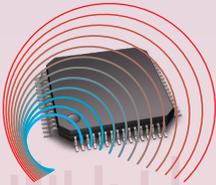
**Lornet36 detector operation is based on the property of semiconductor components to generate a response at the 2d and 3d harmonics when radiated by an RF probing signal.** The detectors analyze the 2d and 3d harmonics response of the radiated objects, which enables a quick and reliable identification of electronic devices and natural oxide semiconductors.
